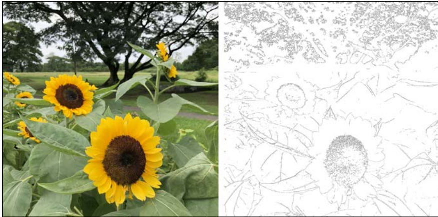
Figure 7.1.1: Example of aligned image pair: left, original image and right, transformed image using a Canny edge detector. Original photos were taken by the author.
